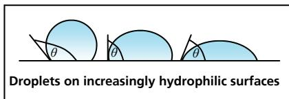
No known material can be used to make a smooth surface with a superhydrophobic contact angle. Some plants overcome this restriction by covering their leaves with tiny bumps. This project looks at plants, like Nasturtium and Lady's Mantle, whose leaves are observed to be superhydrophobic. Water droplets on these plants are nearly spherical.
