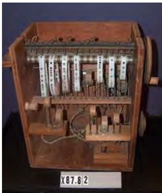
Figure 6. A Number Sieve Machine using 16 mm film (1936). Dimensions: 18 x 19 ½ x 10 ¼ in. Courtesy of the Computer History Museum.
