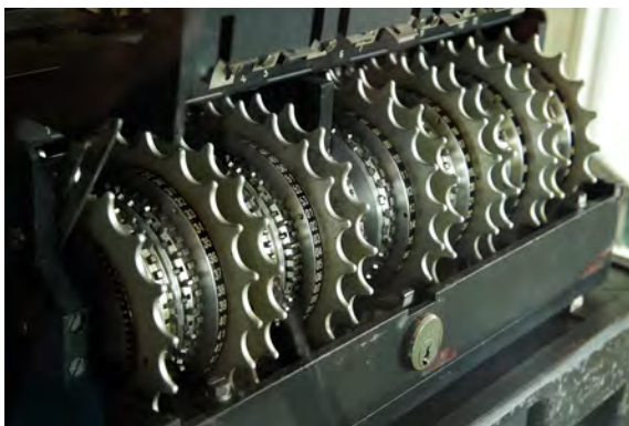
The wheels of a Lorenz machine. (Photo courtesy of The National Museum of Computing www.tnmoc.org .)
