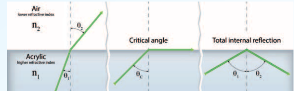
The bending of the light is described by Snell's Law. This equation relates the angle the light beam makes with the boundary between the two materials to the refractive index of the materials.
